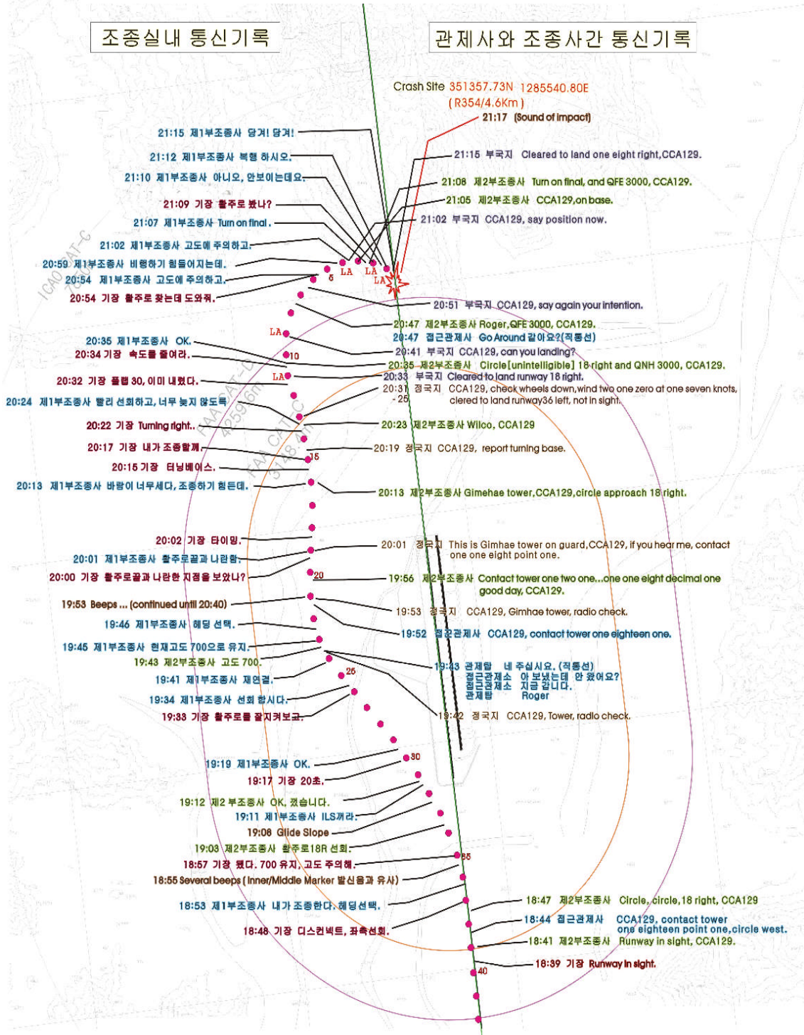
Figure 1-1 CVR & ATC Transcripts Plotted along the Flight Track from the FDR Data (Korean Version)
